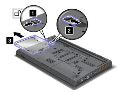
3. Insert the new device firmly into the bay.
